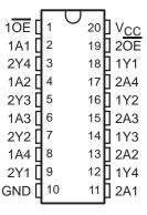
To ensure the high-impedance state during power up or power down,  $\overline{OE}$  should be tied to  $V_{CC}$  through a pullup resistor; the minimum value of the resistor is determined by the current-sinking capability of the driver.
